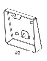
Place Slam Jam bracket (2) onto rim bracket.
